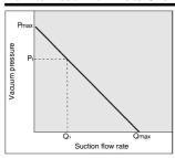
Flow rate characteristics are expressed in ejector vacuum pressure and suction flow rate. If suction flow rate changes, a change in vacuum pressure will also be expressed. Normally this relationship is expressed in eiector standard use.
