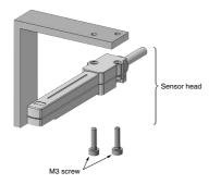
Align bolts with their seating surfaces to mount the sensor head. Mounting it by inserting the bolts from the opposite side may damage the sensor head.
