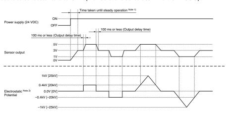
Note 1) The sensor is ready for operation approximately one second after power-on but may provide unsteady readings. It is therefore recommended that the sensor be used more than 10 minutes after power-on.
