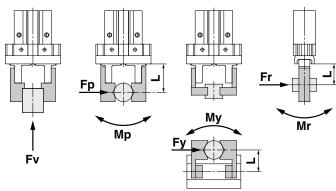
L: Distance to the point at which the load is applied [mm]
