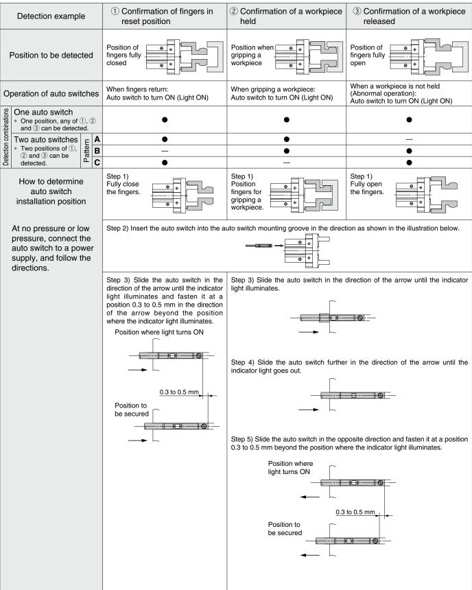
\* • It is recommended that gripping of a workpiece be performed close to the center of the finger stroke.
