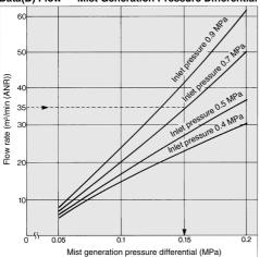
EX: How to obtain the mist generating pressure differential if the flow rate obtaine in 1. above is 35 m³/min (ANR) and the line pressure (inlet pressure P<sub>1</sub>) is 0.7 MPa:
