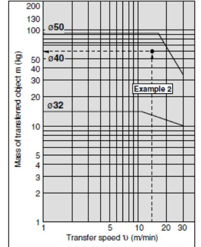
\* Lever-type mass of transferred object and transfer speed graphs (graphs (2) and (3)) show the values at room temperature (20 to 25°C).
