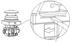
Insert the flat blade screwdriver into the groove.
