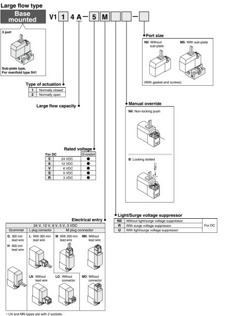
Refer to page 1366 for the different lead wire lengths of L and M plug connectors.
