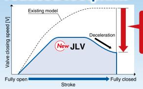
Impact energy when the valve is closed (Proportional to V<sup>2</sup>) DOWN 90%
