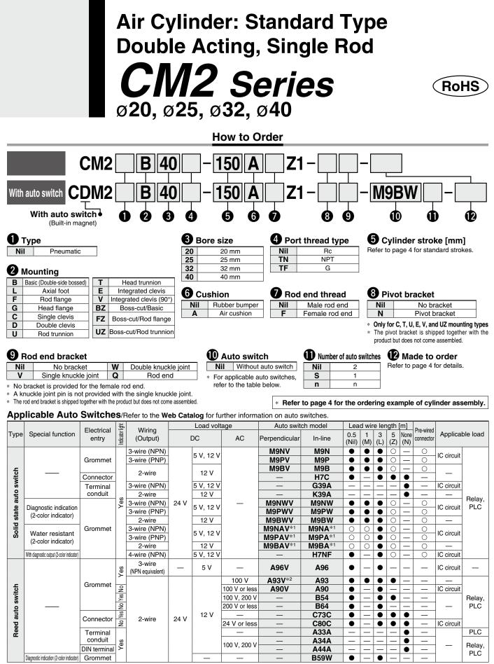
Water-resistant type auto switches can be mounted on the above models, but SMC cannot guarantee water resistance. \*1
