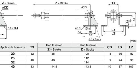
\* A pivot bracket pin and retaining rings are not included with the pivot bracket.
