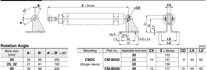
\* A pivot bracket pin and retaining rings are not included with the pivot bracket.
