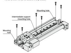
4. When a 25 mm adjustment bolt is selected, the mounting holes will be hidden behind it. Adjust the adjustment bolt after the cylinder
