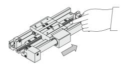
Never disassemble the magnetic component parts (external slider, internal slider) of the actuator (cylinder).
