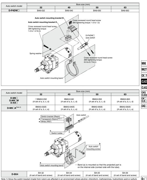
Note 1) Since the switch bracket (made from hylon) are affected in an environment where accord, chloroform, methylamines, hydrochloric acid or sulfur acid is splashed over, so it cannot be used. Please contact SMC regarding other chemicals.
