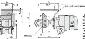
When you attach a dog fitting, be sure to use a knuckle joint, M6 with tap (rod end bracket symbol IA or YA). The dog fitting cannot be attached to the knuckle joint, M6 without tap (rod end bracket symbol I or Y).
