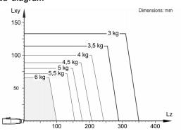
The KR 6 R900 sixx is designed for a rated payload of 3 kg in order to optimize the dynamic performance of the robot. With reduced load center distances, higher loads up to the maximum payload may be used. The specific load case must be verified using KUKA.Load. For further consultation, please contact KUKA Support.
