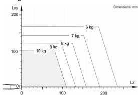
The KR 10 R1420 is designed for a rated payload of 10 kg in order to optimize the dynamic performance of the robot. With reduced load center distances, higher loads up to the maximum payload may be used. The specific load case must be verified using KUKA.Load. For further consultation, please contact KUKA Support.
