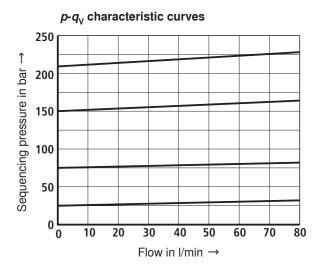
The characteristic curves apply to the pressure at the valve output p = 0 bar across the entire flow range.
