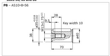
1) Center bore according to DIN 332 (thread according to DIN 13)
