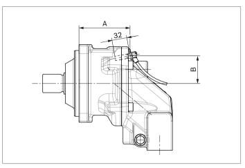
Version "B" A2FE with speed sensor DSA mounted
