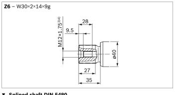
Splined shaft DIN 5480, sizes 56, 63 and 80
