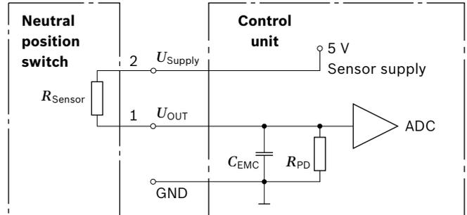
$$U_{OUT} = \frac{U_{Supply} \times R_{PD}}{R_{PD} + R_{Sensor}}$$
