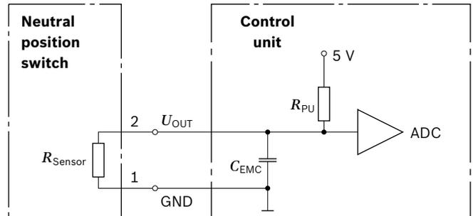
$$U_{OUT} = \frac{U_{Supply} \times R_{Sensor}}{R_{PU} + R_{Sensor}}$$
