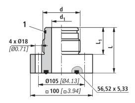
4 x hexagon socket head cap screw, ISO 4762 - M16 x 45 - 10.9 included in the scope of delivery
