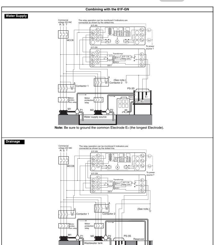
Note: Be sure to ground the common Electrode E3 (the longest Electrode).
