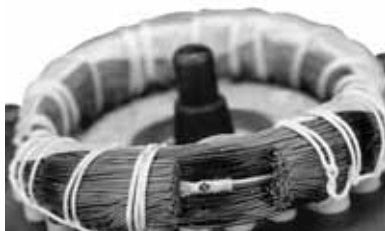
Fig. 40 PTC sensor incorporated in windings
