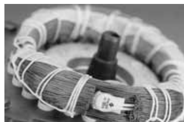
Fig. 42 Thermal switch incorporated in windings
