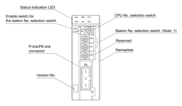
Note: 1) Only PL is used for the P-link module. (0 to F)
